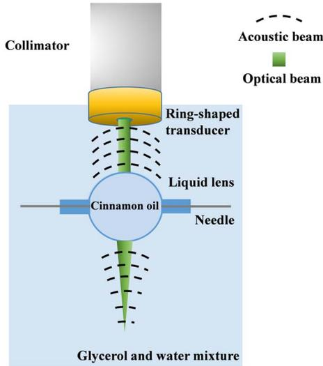
Fig. 2. Schematic of the compact ORPAM imaging probe.
