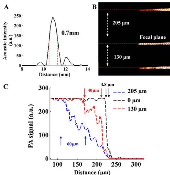
Fig. 4. A, 1D profile along the dashed white line across the acoustic focal point shown in Fig. 3B; B, B-scan images of the blade in the focal plane. 130 and 205  $\mu\text{m}$  off the focal plane; C, 1D profile along the red dashed line shown in Fig. 4B.
