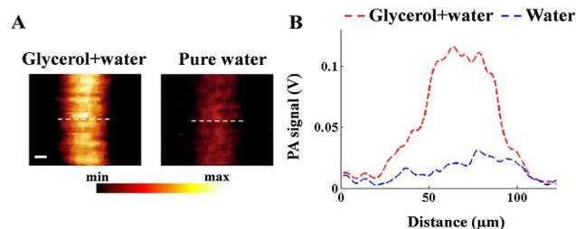
Fig. 5. A, MAP of human hair with and without acoustic focusing; B, 1D plots along the dashed lines in Fig. 5A. Scale bar: 20  $\mu\text{m}$ .
