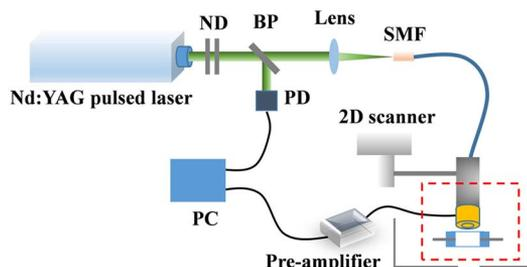
Fig. 1. Schematic of the ORPAM imaging system. ND, neutral-density filters; PD, photodiode; BP, beam splitter; SMF, single-mode fiber.
