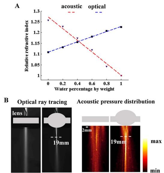
Fig. 3. A, acoustic and optical relative refractive index versus weight percentage of water in the mixture; B, optical rays and acoustic pressure distribution when the lens was flat and fully infused.
